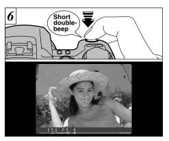
When you press the shutter button down halfway, the camera emits a short double-beep and focuses on your subject. At that point, the AF frame on the screen becomes smaller and the camera sets the shutter speed and aperture.
